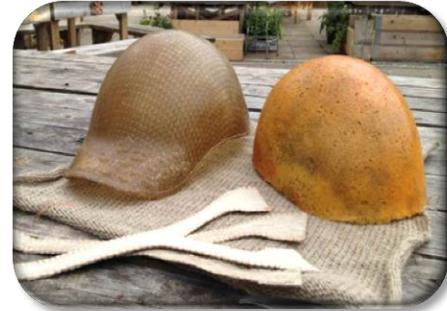
**Duo Lin cycle helmet incorporating a tough knitted flax woven outer resin shell (left) and dense bio-resin foam core interior (right)**
