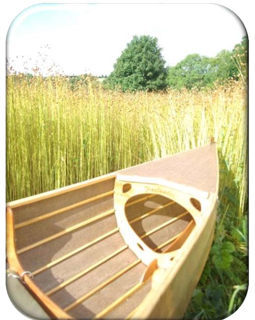
Flax fabric is coated with linseed epoxidised resin & cured under UV sunlight to waterproof the craft
